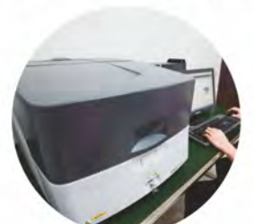
Energy dispersive X-ray fluorescence spectrometer To detect the harmful materials, according with the demand of EU standard
